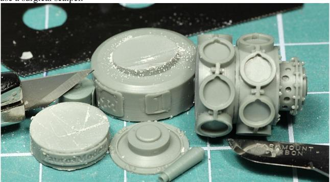
Connect the crankcase elements (2) and (12) using a two-component epoxy glue (this leaves some time for the proper positioning). Attach the shaft (3).
