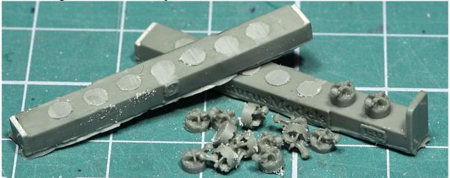
Next put the heads into the holes in cylinders. Use two-component glue, in order to
